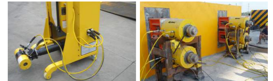
▲ Matching big diameter pipe orifice adjustment of orifice calibration machine. ▲ Synchronous tensioning of high-speed rail box girder.
