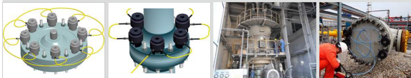
▲ Bolt synchronous pre-tightening of pipe flange bolt. ▲ Bolt synchronous tensioning and pre-tightening in series. ▲ Vertical mill foundation bolt pre-tightening in cement plant. ▲ Pressure vessel bolt synchronous pre-tightening in refinery.
