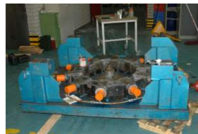
▲ Synchronous locking of cable of cable-stayed bridge in bridge girder construction.
