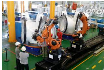
▲ Assembly of wind turbine hub.
