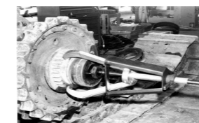
▲ Bearing disassembly for mining machinery maintenance.
