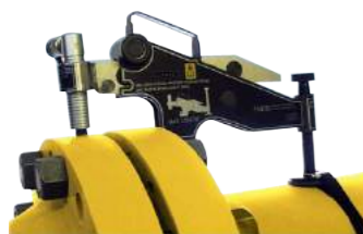
▲ Petroleum pipeline flange adjustment.
