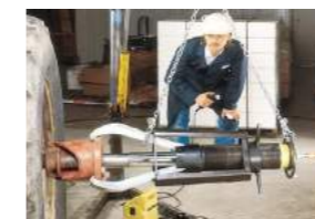
▲ Tyre bearing disassembly for large mining machinery.
