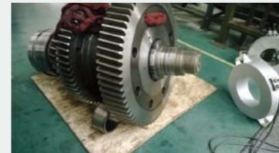
▲ Bearing heating and disassembly for large gear case.
