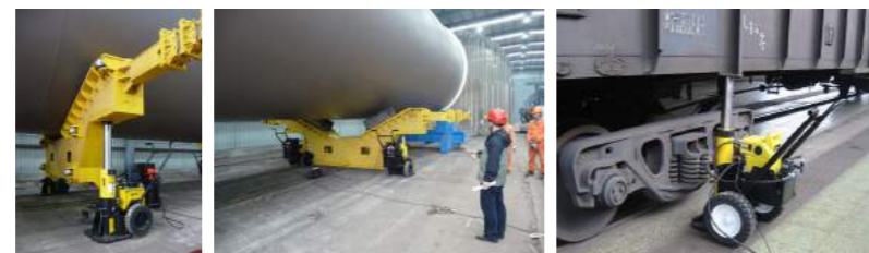
▲ Synchronous lifting of large tank. ▲ Synchronous lifting of large pressure vessel. ▲ Locomotive repairing and lifting.
