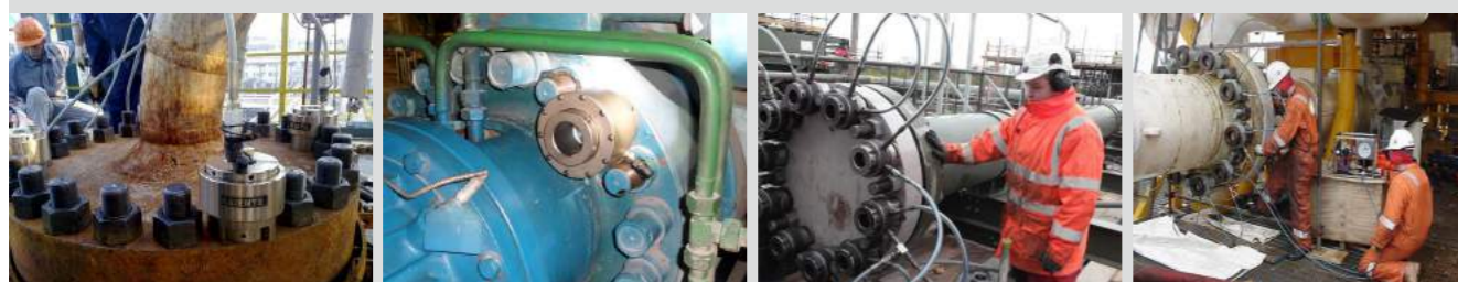
▲ Pressure vessel bolt synchronous pre-tightening in chemical plant. ▲ Bolt pre-tightening of large electric motor in thermal power plant. ▲ Bolt synchronous pre-tightening of pipe flange bolt. ▲ Pressure vessel bolt synchronous pre-tightening in steel mill.
